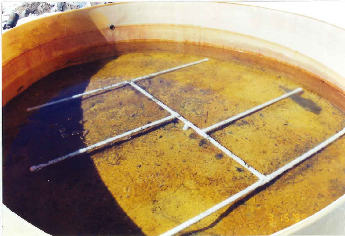
Photo 4. Pilot scale vertical flow tank constructed using composted biosolids and #9 limestone. Overdrain lattice work distributes acid mine drainage received by feeder pipe at center. Jennings Environmental Education Center, Brady Township, Butler County, PA. (3/15/1999)
