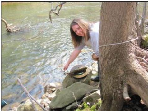
*A horizontal datalogger installation*
