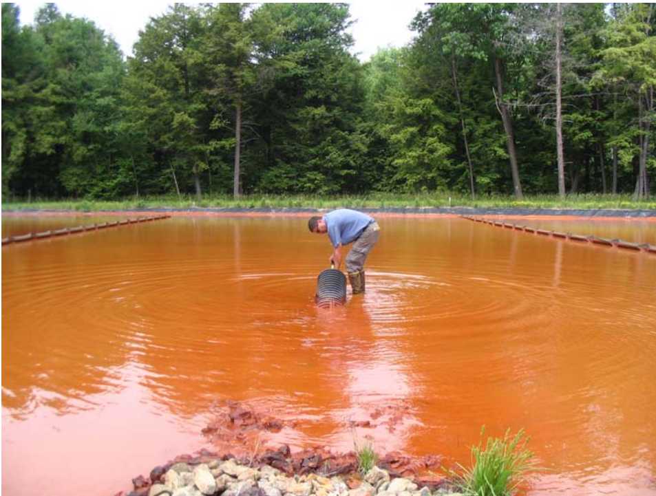
Photo F. Measuring flow from the underdrain discharge.
