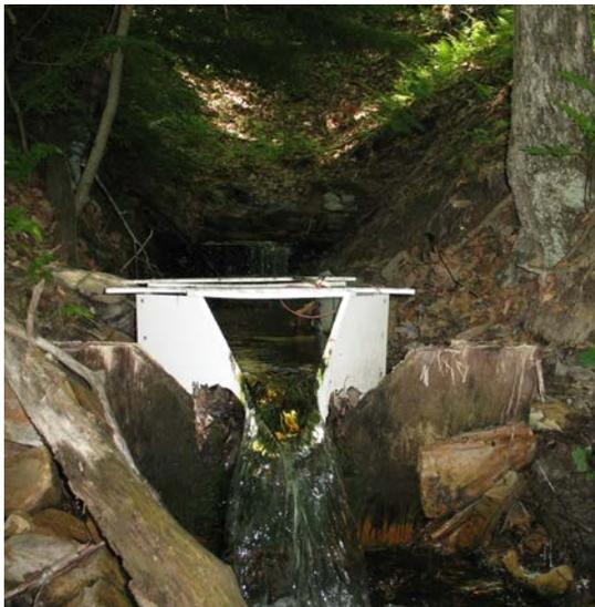
Weir at KC204 discharge to measure flow from the deep mine.
