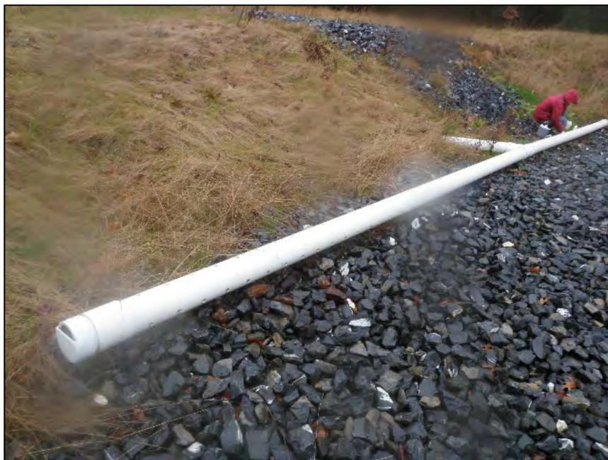
View of Missy Reckner of the Kiski-Conemaugh StreamTeam collecting water samples at the inlet distribution pipe (Top) and of the entire Weaver Run D8B limestone bed (Bottom).
