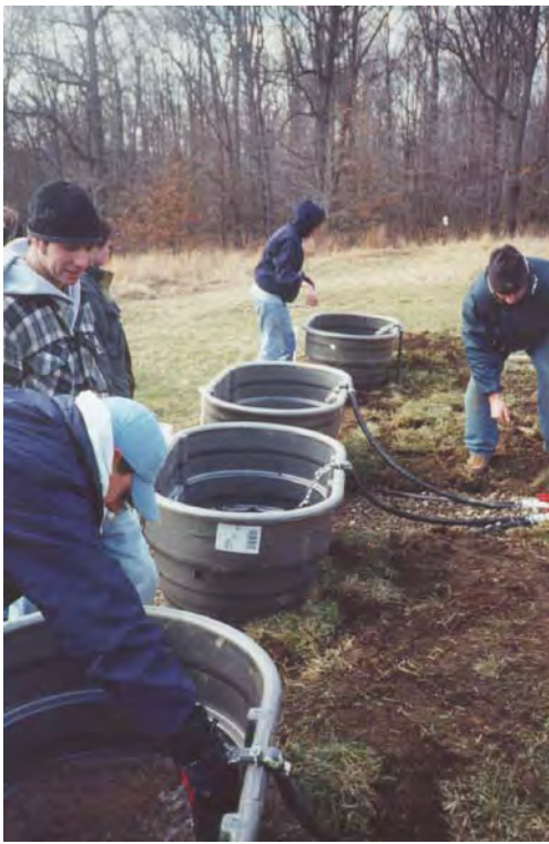
Left: Westminster College students setting up the small-scale vertical flow pond test tanks. Right: Westminster College students performing their initial 24-hour sampling period.
