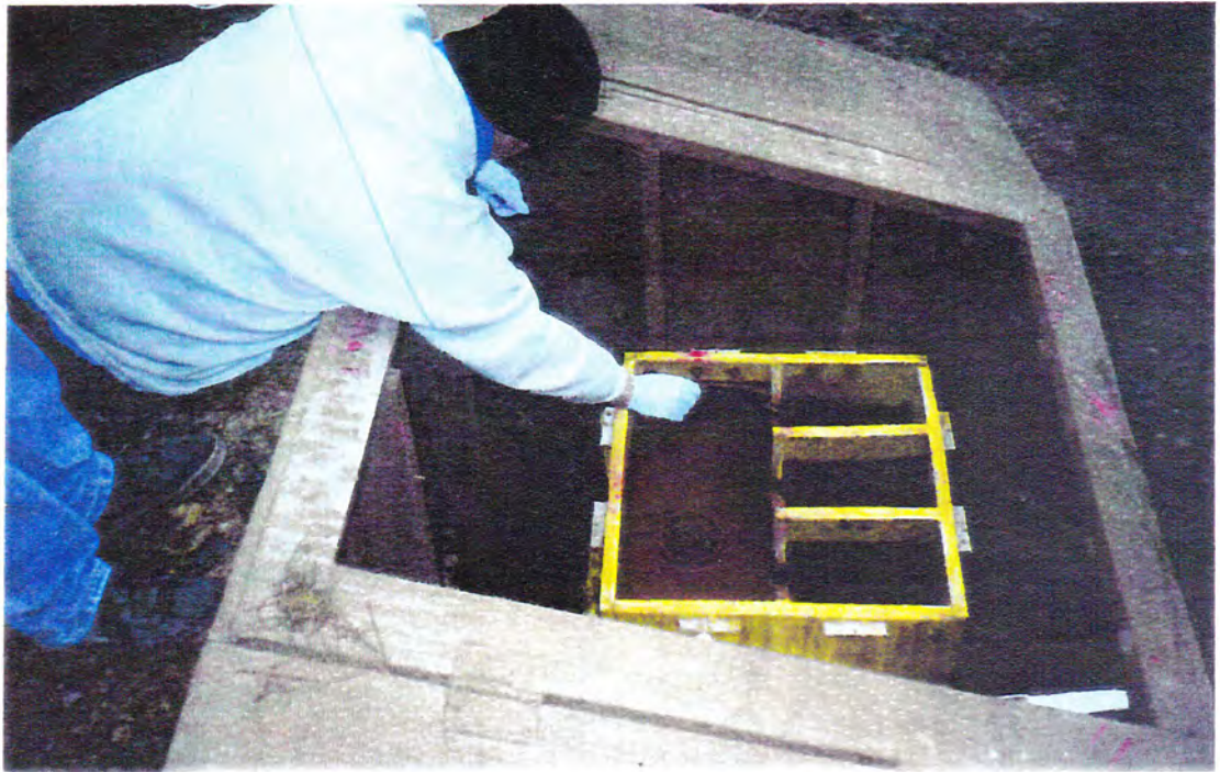
VOLUNTEER KITTY PEART participating in a dye test to study the effectiveness of the water distribution system at the Jennings Environmental Education Center. Home school students and volunteers have conducted these tests to study the innovative techniques used for the passive treatment of abandoned mine drainage at Jennings.
