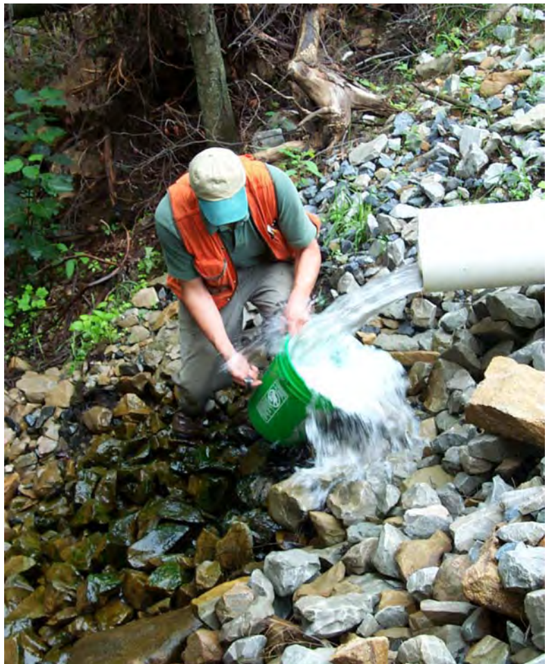
The effluent of the B1B3 Vertical Flow Pond flows through the B1B3 Settling Pond/Wetland before entering the Horizontal Flow Limestone Bed (above).
