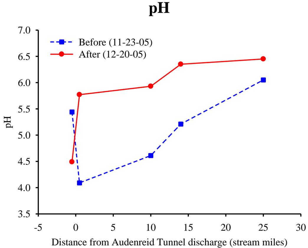
Figure 1. pH at various sampling points (stream miles) along the Cattawissa Creek before and after construction of the Audenreid Treatment System.
