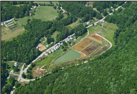
Phase I lowered the mine pool by using an innovative technology called in-seam directional drilling. Through in-seam directional drilling, the original discharge was relocated to an area close to where land had been acquired for the construction of a passive treatment system.
