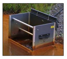
A flow in cubic feet/second is calculated where H = height of water flowing through weir in feet and W = width of weir in feet (2.64' for Agri-drain Inlet Control Structure)
