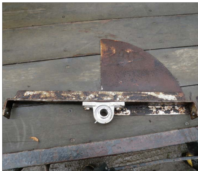
Top Left & Right: The cyclone screen being cleaned to allow flow to the Oxid Limestone Drain. Bottom Left: The siphons which may be disabled as needed to allow the cyclone to function properly. Bottom Right: The bearings for the cyclone screen were replaced.
